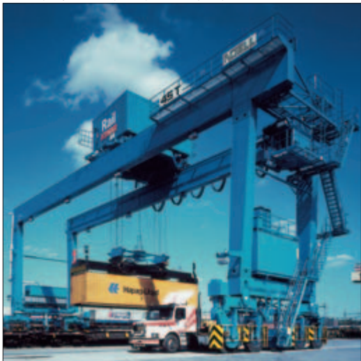
Security in logistics: Positioning and track guiding using transponders (on the chassis and within the bridge; for identification of vehicles (e.g. trucks))
