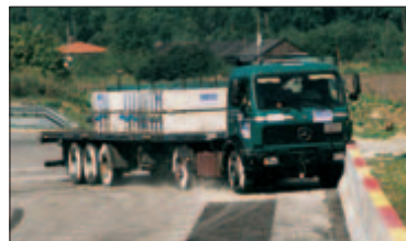
Optical track guiding using colored tape fixed to the ground suitable for low-cost or temporary installations (e.g. vehicle cranes)
