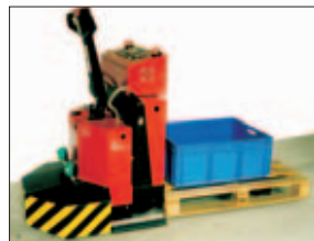
Extremely effective: inductive track guiding of container transport
