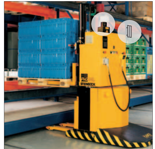
Laser Scanner for independent navigation (indoor AGV (shown))
