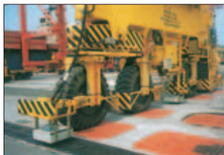
2 dimensional positioning and track guiding using transponders for rubber drive off the drivers (shown: Rubber Tired Gentry Crane RTG)
