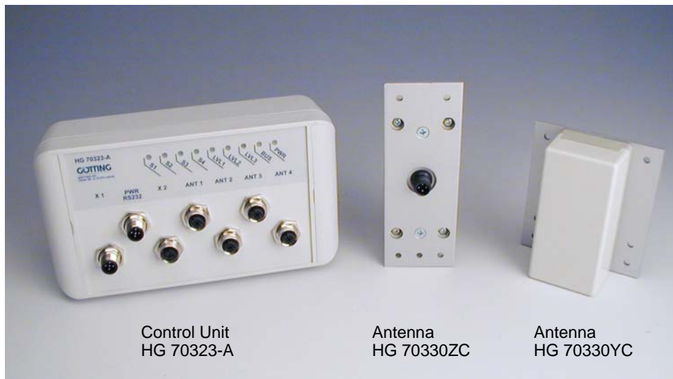
Figure 1 Inductive Proximity Warning System
