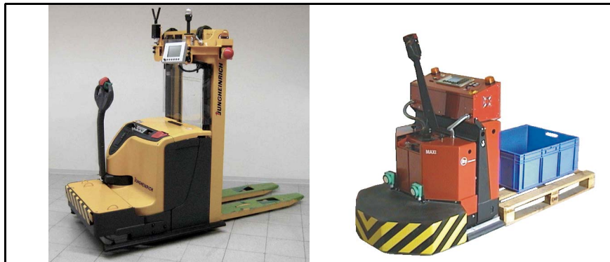
Figure 5 Examples of driverless vehicles with transponders
