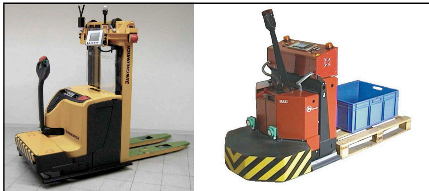
Figure 2 Examples of AGVs using RFID systems
