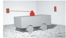
Most vehicles used for internal transportation are more or less guided by a fixed system. This includes railbound systems as well as systems that are guided by an inductive wire. Using inductive transponders within the track already offers more flexibility. However, navigation via laser scanners has proved to be even more advantageous.
