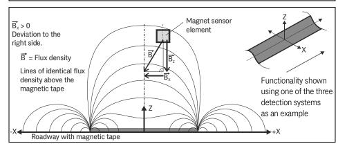
The magnet sensor HG G-19600ZA detects the magnetic field above a magnetic tape in horizontal and vertical direction and continuously calculates the actual deviation diagonally to the direction of travel. The deviation is then output as an analog voltage.
