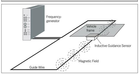
The inductive guidance sensor HG G-19370 / HG G-19380 is used for the inductive track guidance of Automated Guided Vehicles (AGV). Up to 5 different guide wire frequencies may be detected and evaluated simultaneously. Alternatively a ground installation for the contact-less inductive energy transmission with two wires (energy track) can be used for the track guidance.
