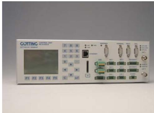
tion is included. For all other Guidance Solutions, the Navigation Controller processes the received position information together with the received information about the vehicle velocity (e.g. via encoders).
