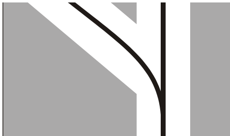
Example of an optical track branching
