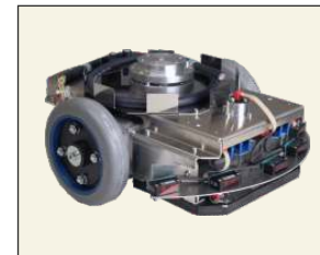
Drive-Steering Module for AGV
