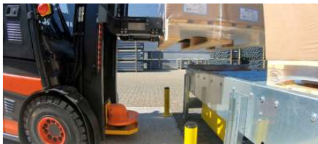
Figure 2: Load transfer to conveyor with bearing marks
