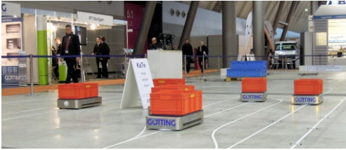
HG 22710: Punctiform contactless energy transfer up to 1.3 kW, also for small vehicles
