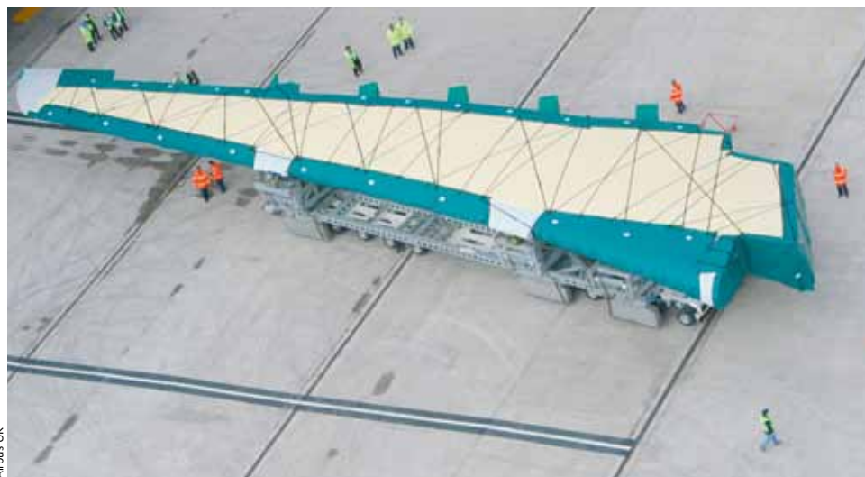
Bottom: Inductively-guided, heavy-duty AGV transports vast aircraft wings
